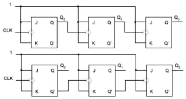
2. Design a **Mod-5** asynchronous counter. A Mod-5 counter counts **0-1-2-3-4-0**. First determine the number of flip-flops, and for an up counter. Then, form the resetting mechanism for the output of 6. You can use the CLEAR input of the flipflops. Construct the circuit, and check your results.
