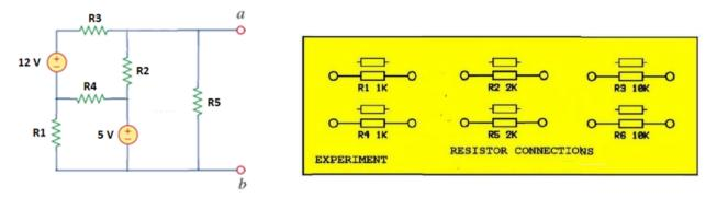
Implement the given circuit and then short citcuit terminal a-b. Measure the short circuit current *i<sub>ab</sub>*.
