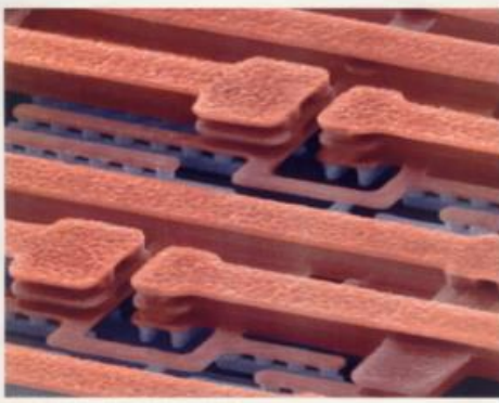
Upclose (side) view of the individual wires in a typical integrated circuit
