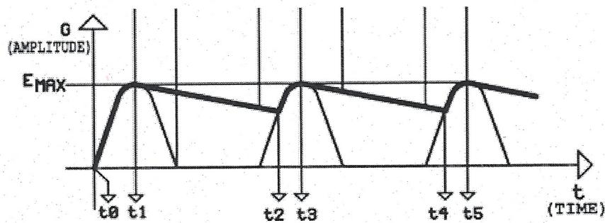
(5p) If the value of C increases, how does the peak to peak value of ripple voltage of E0 change? Why?
