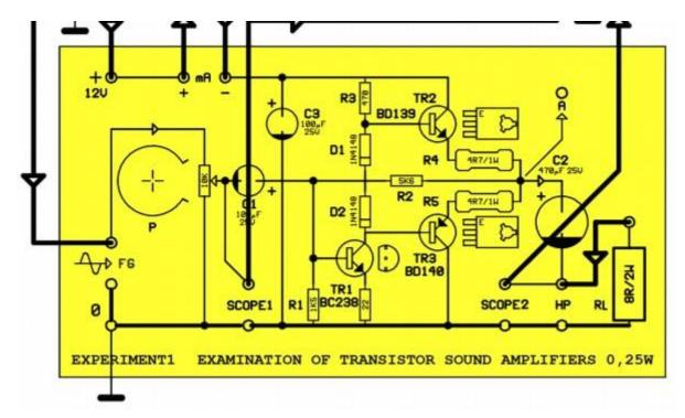
hFE=100, hfe=100, IC>>IB, ic>>ib 1-) Analyze this circuit for DC. Find IC, IB for each transistors.
