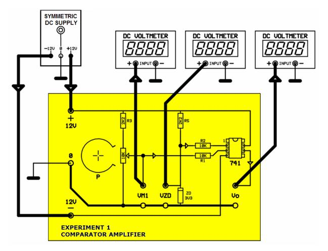
**1-** Apply power to the circuit. Measure the voltage (**VZD**) across the terminals of the zener diode connected to the circuit. What is that voltage called?
