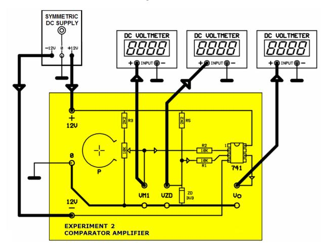
**1-** Apply power to the circuit. Measure the voltage (**VZD**) across the terminals of the zener diode (between the points A-O) connected to the circuit. What is that voltage called?
