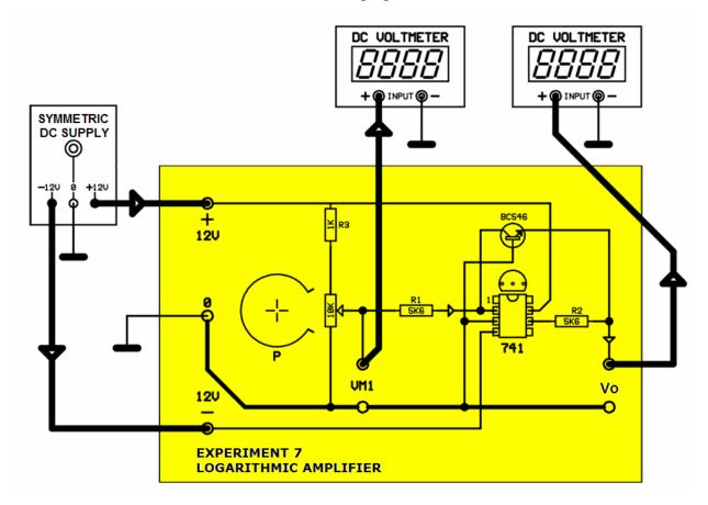
**1-** Apply power to the circuit. Adjust the input voltage V1 to the values given in table 1 by using the potentiometer P. Take note of the output voltage in each step.
