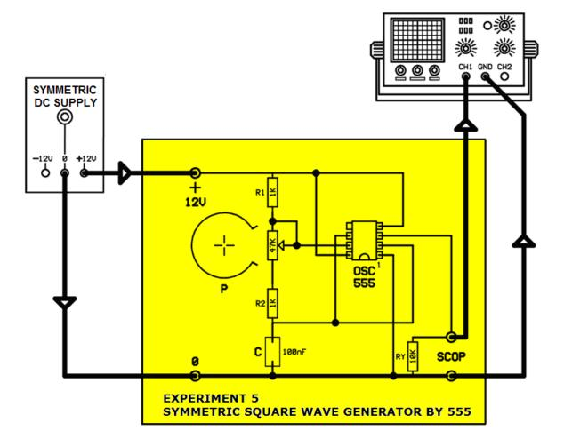
**1-** Apply power to the circuit. Set the potentiometer to its maximum resistance position (middle pin is up). Measure the amplitude, the frequency and duty cycle of the signal on the oscilloscope screen.
