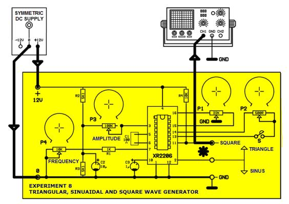
**5-** Set the P4 potentiometer to minimum and maximum. Measure the frequency band of the circuit?
