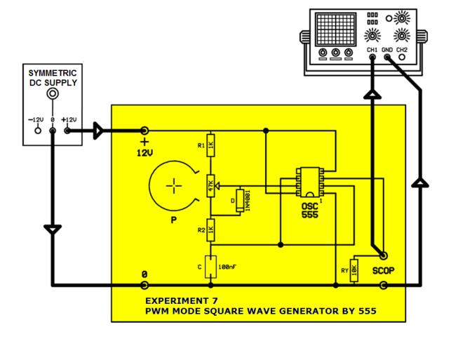
**1-** Set the potentiometer to the mid-value. Apply power to the circuit. Define the output signal. Measure the amplitude of the output signal? Draw the shape and measure the duty cycle of the signal
