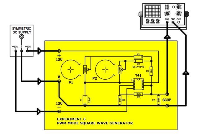
**1-** Apply power to the circuit. Measure the amplitude of the output signal. Why is that value obtained? Draw the shape and measure the duty cycle of the signal.
