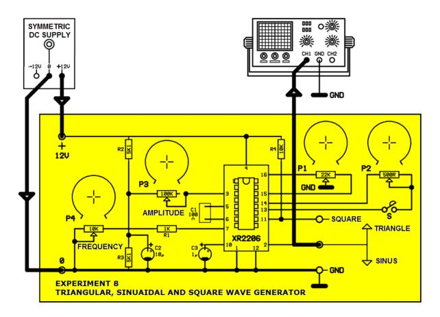
Set the oscilloscope to AC. Set the sine/triangular select pin to sine state (switch pin is down). At this moment, the switch is closed. Apply the power to the circuit. Define the waveform in the oscilloscope? Draw the signal.
